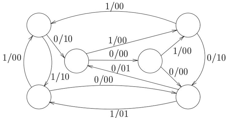
Figure 2: Rate 1 : 2 six-state encoder for the  $(2, 7)$ -RLL constraint.
